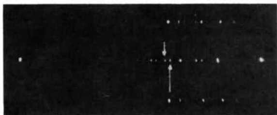
Fig. 3. An a -axis 15^\circ -oscillation photograph of a \text{PbI}_2 crystal, showing reflections of 12R_R and 12R_0 . Other conditions as for Fig. 2. The positions of one reflection each of 12R_R and 12R_0 are indicated by arrows pointing upwards and downwards, respectively.
