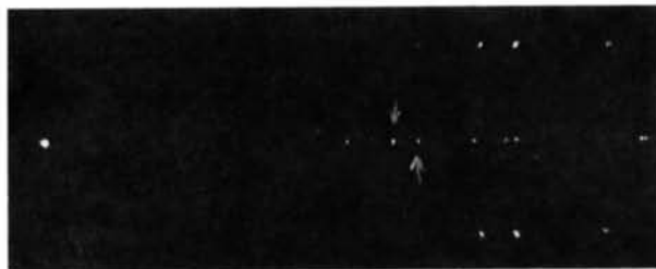
Fig. 5. An a -axis 15^\circ -oscillation photograph of a \text{CdBr}_2 crystal showing reflections of 6R_R and 6R_0 . Other conditions as for Fig. 2. The positions of one reflection each of 6R_R and 6R_0 are indicated by arrows pointing upwards and downwards, respectively.
